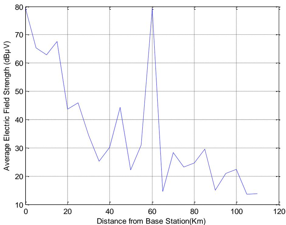
Figure 4: Signal Propagation Curve for Yenagoa-Nembe Route
