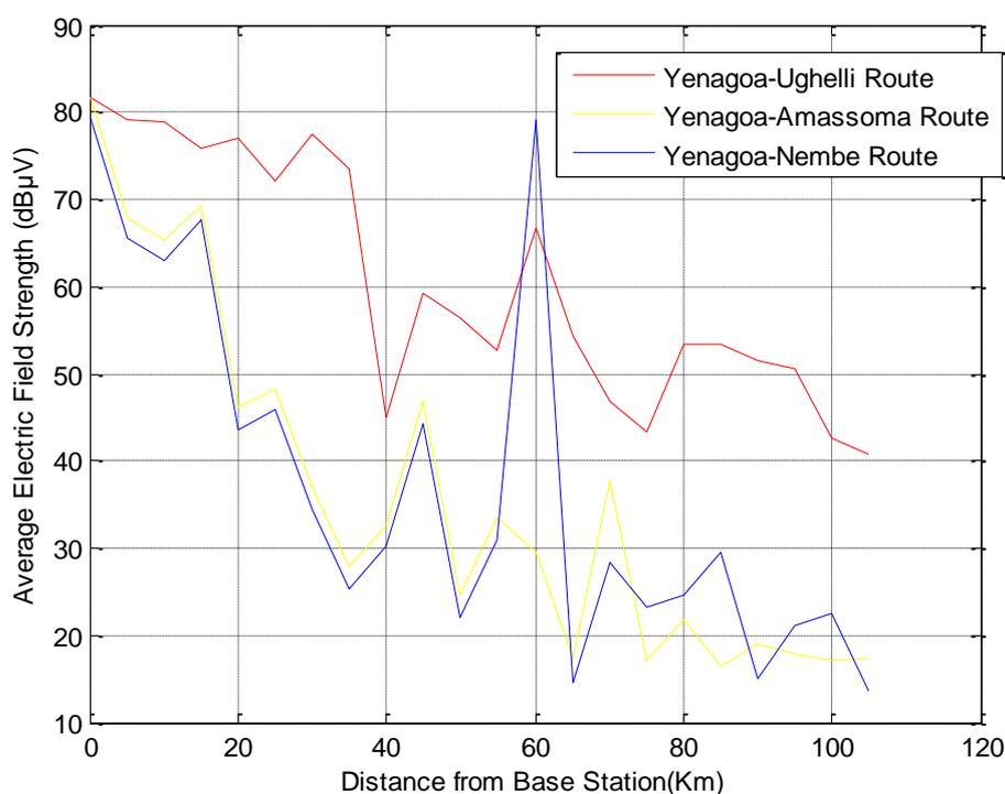
Figure 5: Signal Propagation Curve for the three Routes
